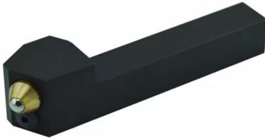
Fig. 2: A rigid burnishing tool was used in this study, with a tungsten carbide ball, 30° bend tip, and 20×20 mm shank.
